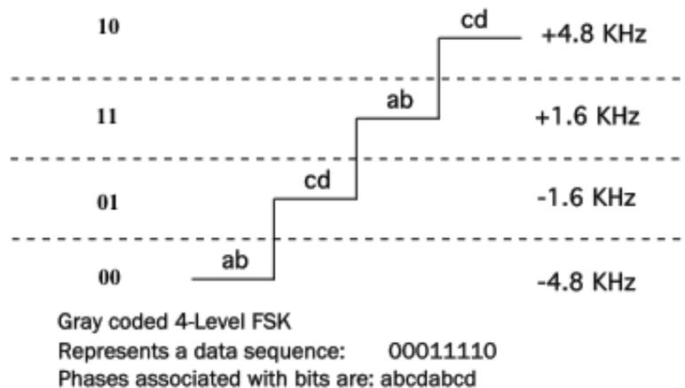
Conceptually, the modulation is developed by passing Non-Return to Zero (NRZ) Pulse Amplitude Modulated (PAM) square waves through a 10th order low pass Bessel filter with a 3 dB point of 3.9 kHz and sending the resultant symbol stream to a frequency modulator at the carrier frequency. The same low pass break point is used for both baud rates. The Bessel filter is used for its linear phase characteristics, which is desirable in data transmission applications.
