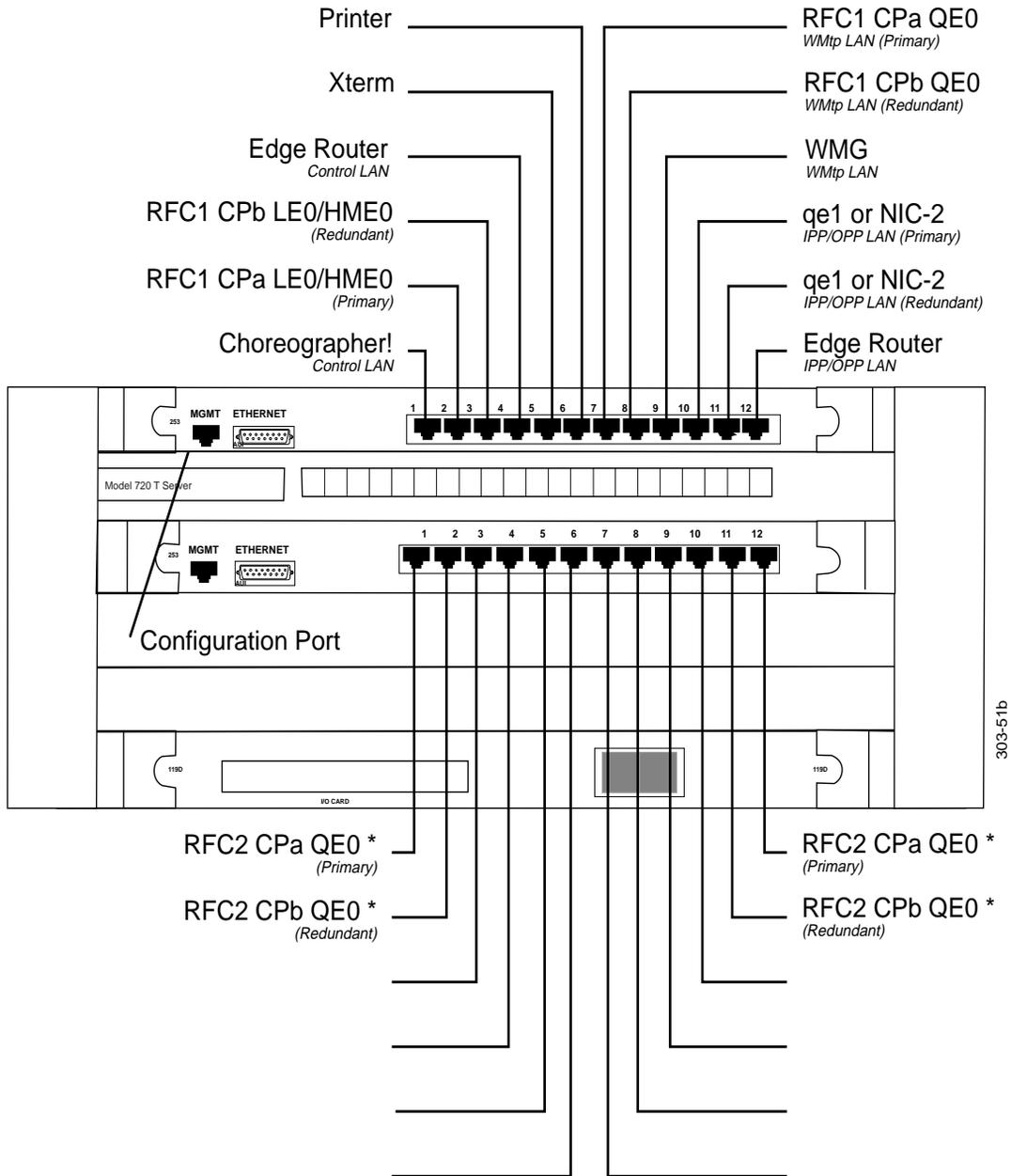
Figure 4-4: Ethernet Hub—Typical Connections
