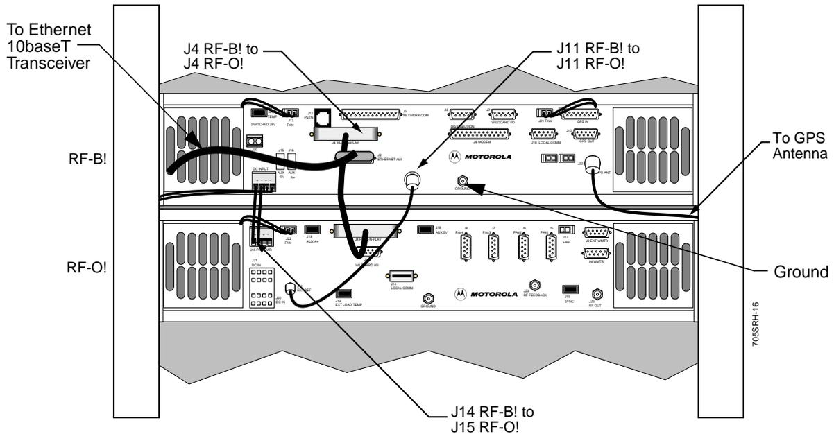
Figure 4-3: RF-B! Transmitter Controller Cabling (Rear View)
