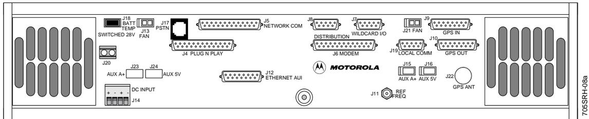
Figure B-1: RF-B! Transmitter Controller Back Panel
